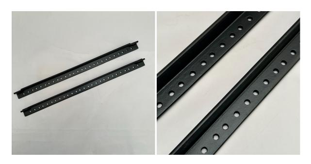
**Step 5:** Before fastening the Allen bolts at the frontend, fix the Rack Mount attachment on the right and left ends of the Interconnectors (#3) as shown in the figure down below.
